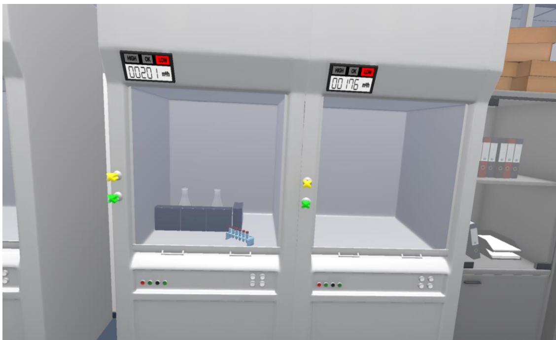
Figure 7: air-flow rate too low (Scenario 1b)
