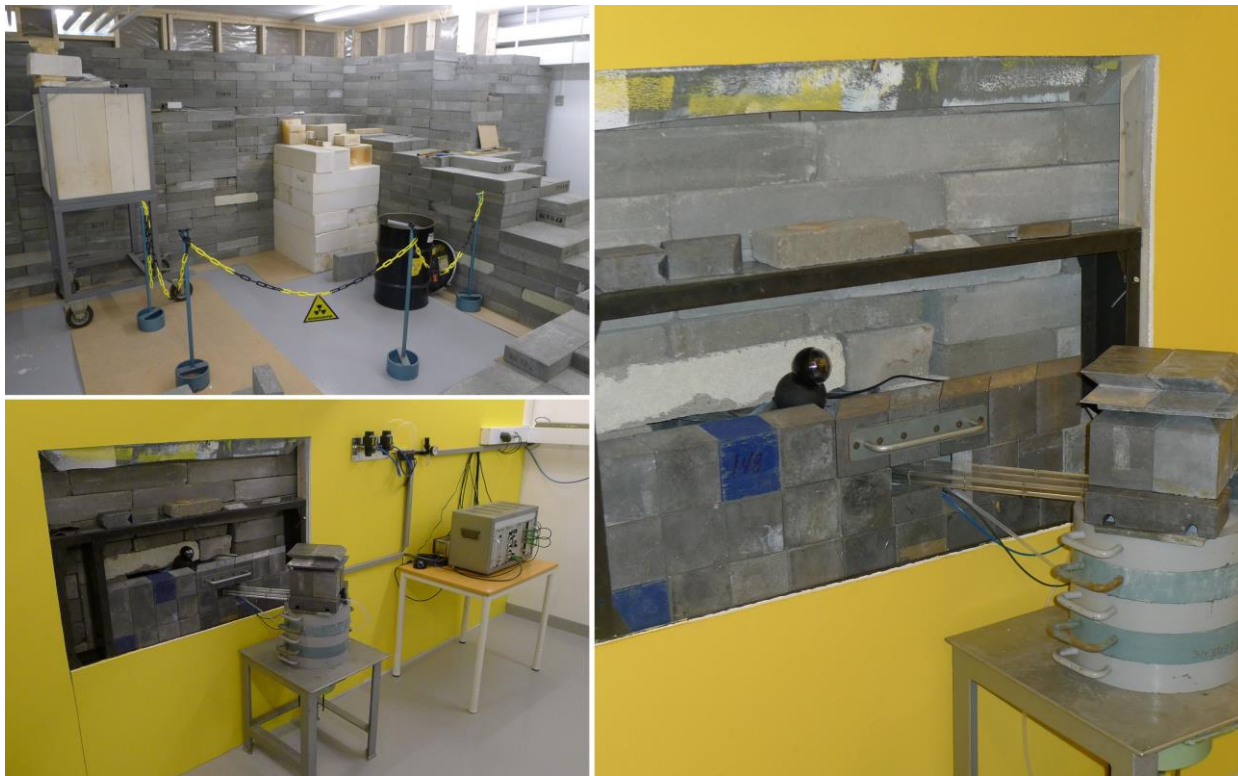
Picture in upper left corner shows the shielding for the ^{238}\text{Pu/Be} n-source. The transport slide comes through the 1 m thick concrete wall and ends inside the pile with boron paraffin. The n-source is placed under the slide and surrounded by about 20 cm of pure paraffin in all directions. On the other side of the concrete wall is the detector inside its lead shielding, as can be seen in the two other pictures.
