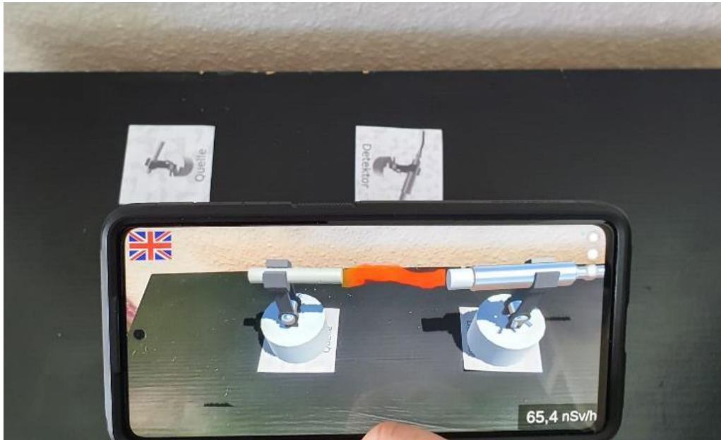
Figure 1 General experimental set up to determine the range of beta radiation in the augmented reality application. In the background one can see the image markers on a table to set up the experiments.
