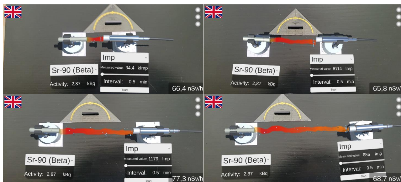
Figure 8: Example setup for taking a series of measurements to investigate distance,, which beta radiation travels in air. Distance between image markers from source and detector: 7 cm (top left), 13 cm (top right), 18 cm (bottom left), 26 cm (bottom right).
