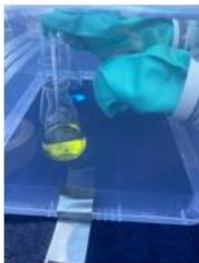
Figure 3: Glove box set up, note the tape to hold it in place on the table
