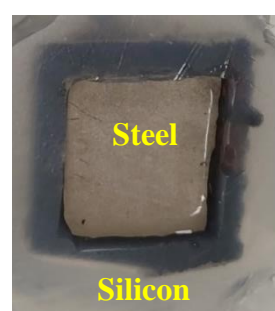
Stainless steel embedded in silicon and decontaminated using the CORD method.
