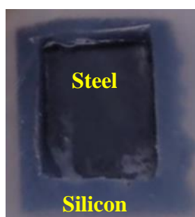
Oxidized stainless steel embedded in silicon and showing a black oxidation layer.
